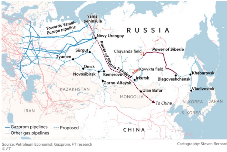
Figure 3.1 - Russian pipeline infrastructure
